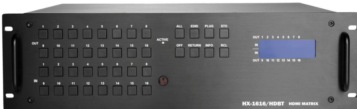
Figure 5-3 HX-1616 Front Panel for 16 Output/Input Keys
