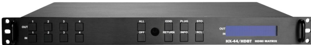
Figure 5-1 HX-44 Front Panel for 4 Output/Input Keys
