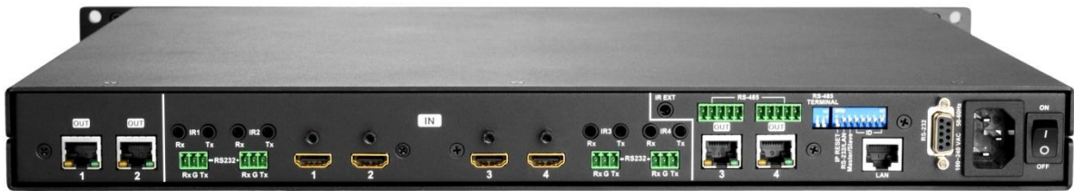
Figure 5-4 HX-44 Rear Panel for 4 Output/Input Jacks
