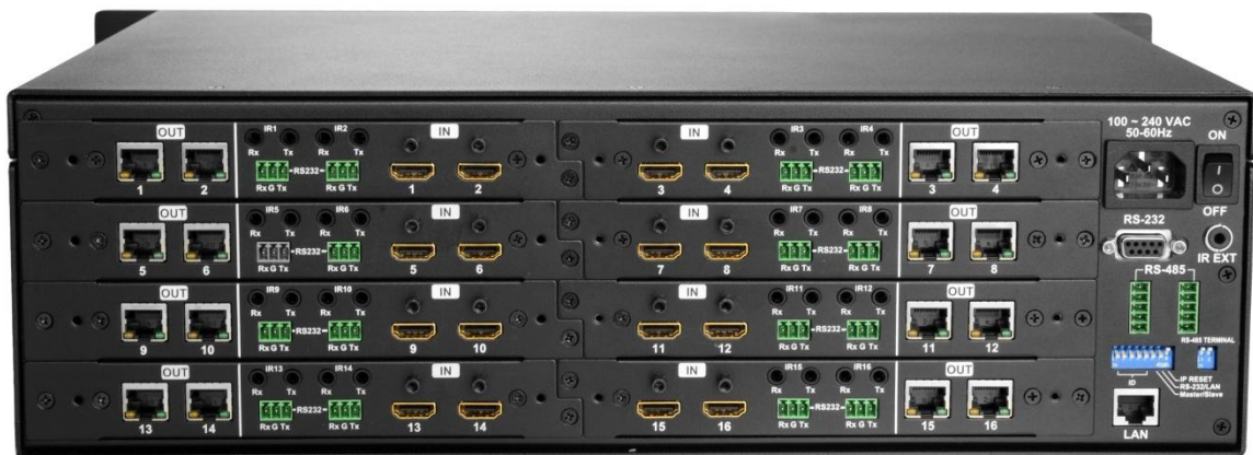
Figure 5-6 HX-1616 Rear Panel for 16 Output/Input Jacks
